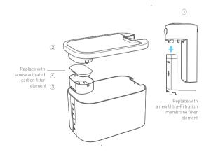
A. 1. Remove the main pump. 2. Fountain Tray. 3. Filter Holder and, 4. Filter.
