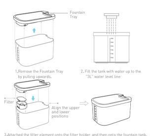
Align the upper and lower holders of the tray with the water storage tank to cover it
